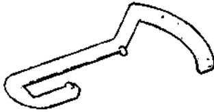
35-660040/810-5 Elevator Check Fixture L.H. 35-660040-1/810-5 Elevator Check Fixture R.H.
